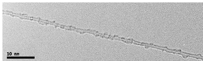
Fig. 4. TEM of functionalized, surfactant-free SWNT deposited from chloroform solution. Reproduced from [83] with permission.
